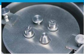
**SEHO SelectFlux**. Selective flux application in wave soldering processes. Your advantage? Minimal consumption and almost no soiling.
