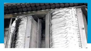
Automatic Nozzle Height Adjustment. In up to 16 different sectors of an assembly, the height of the soldering nozzles can be adjusted individually, controlled by the software, in order to always have the optimal distance between the circuit board and the soldering nozzle, depending on the product.
