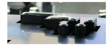
Automatic Ultrasonic Nozzle Cleaning. Forget the time-consuming, manual cleaning of miniwave soldering nozzles or aggressive chemicals: SEHO's ultrasonic nozzle cleaning does this automatically and in an environmentally friendly way for you.
