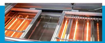
**Pulsar Preheat.** Innovation made by SEHO. The pulsar preheating from SEHO is full of intelligent power and enables the cost-effective and energy-efficient high mix - high volume wave soldering process.
