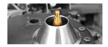
Innovative Multiwave Soldering Processes. Product-specific multi-nozzle soldering tools ensure short cycle times in productions with high throughput and low variety of assembly types. SEHO's soldering nozzle design guarantees optimal energy transfer resulting in excellent hole fill even with high-mass assemblies and demanding geometries.
